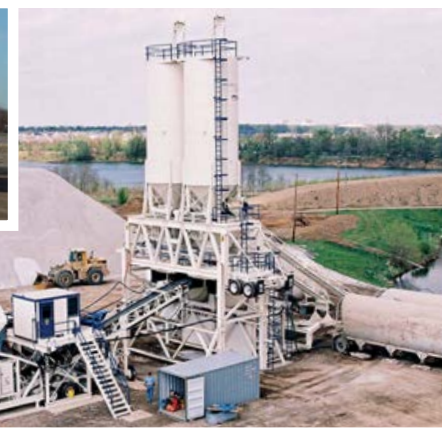
Captions Top left: Ranger 12 with bag style dust collector. Far left: 'Johnson' mixer and frame. Left: Ranger 12 showing an optional elevated control house. Above: Aggregate section with charging conveyors from both sides.
