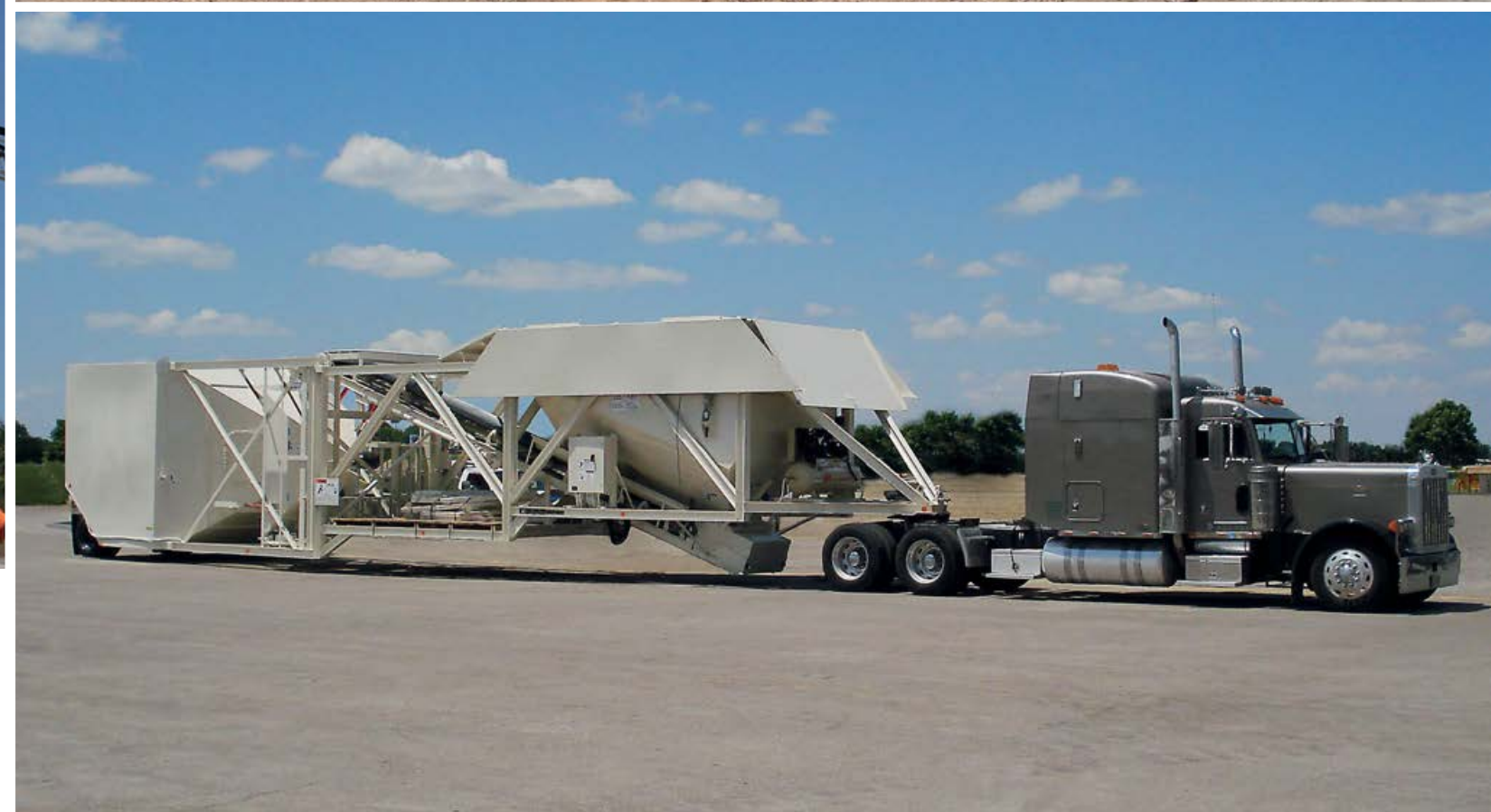
Captions Opposite top: Bandit 12 with bin charging conveyor. Opposite bottom: Bandit 12 folded for transport. Above left: Cylindrical compartmentalized cementitious materials silo. Above: Bandit 12 with multiple cement and other cementitious silos and aggregate bin extensions.
