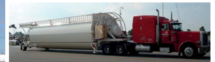
Captions Top left: R1600 59 ton self-erecting silo in transport configuration. Left: R1600 silo coupled with Rustler 12 creating a drive through for trucks. Above top: Vertical pig 'farm' for large airport construction job. Above: 4,665 ft 3 (132 m 3 ) capacity vertical pig being transported.
