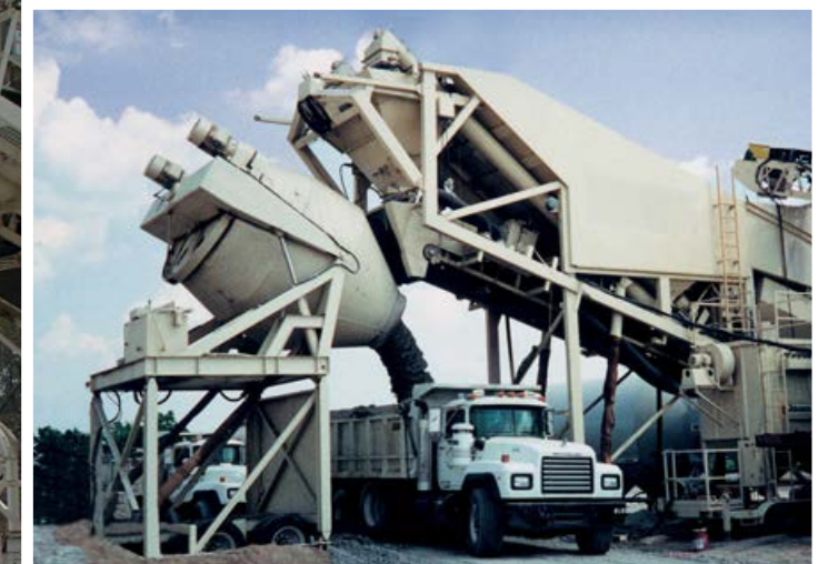
Captions Opposite top: Unirover plant showing optional steel foundation pads. Opposite bottom: U12 plant setup and ready to go. Above: Unirover 'Johnson' mixer discharging into end dump truck. Left: View showing the 'Johnson' mixer elevated.
