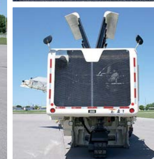
Captions Top: The RM-9 features 950 hp and cutting widths to 12 ft 6 in (3810 mm). Opposite left: 43 in (1067 mm) conveyor has 60° left and right swing. Left middle: Hydraulic rear door allows ground access to cooling package. Left: Gullwing doors provide excellent access to power pack components. Above: Cutter door gives great access for tool replacement.
