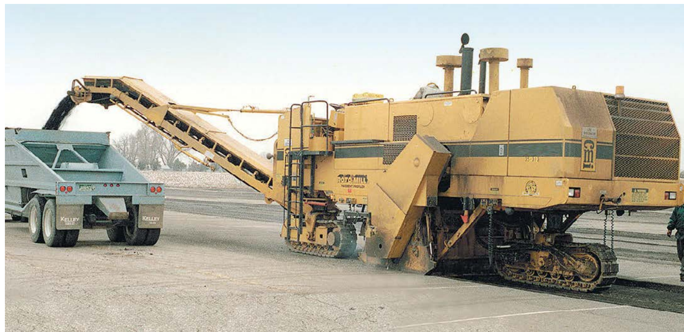
Captions Above & right: The twin engine configuration of the RM-12 allows cut widths up to 14 ft (4.25 m).
